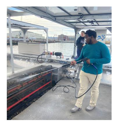
Use automatic or manual Spray Wash System for cleaning and biofouling control.
