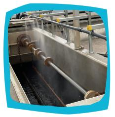
SOPS can now come with an authmatic spray wash system to clean the baskets as they rotate.
